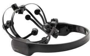
FIGURE 3. Emotiv Epoc headset with 14 channels.
