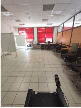
Fig. 2. Experiment 1 set up. Subjects had to stop the wheelchair in the 2 predetermined stop positions in order to evaluate the ability of the BCI-controlled wheelchair to stop with precision. The two designated stopping points are demarcated by distinct X-shaped markings on the floor.
