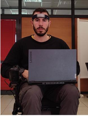
Fig. 1. System Overview. The Muse S connects with the computer via Bluetooth and the computer connects with the wheelchair via USB.
